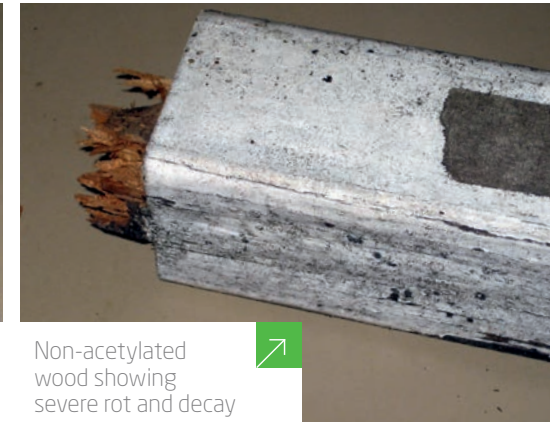
Non-acetylated wood showing rot and decay
